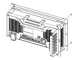
Get encased in the cabinet: Mount the assembled instrument and rack into a standard 19-inch cabinet by using six M6 screws and six M6 square nuts.
