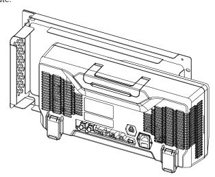
3. Install the right plate: Attach the right plate to the right edge of the front plate, then fasten them with two M4 screws.
