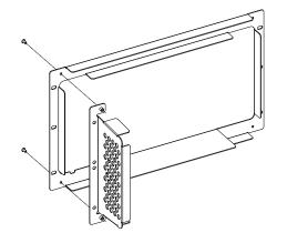
2. Place the instrument: Place the instrument into the frame set up by the front plate and the left plate.
