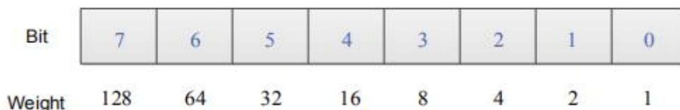
Figure 2.5 Relationship between the bit and the weight
