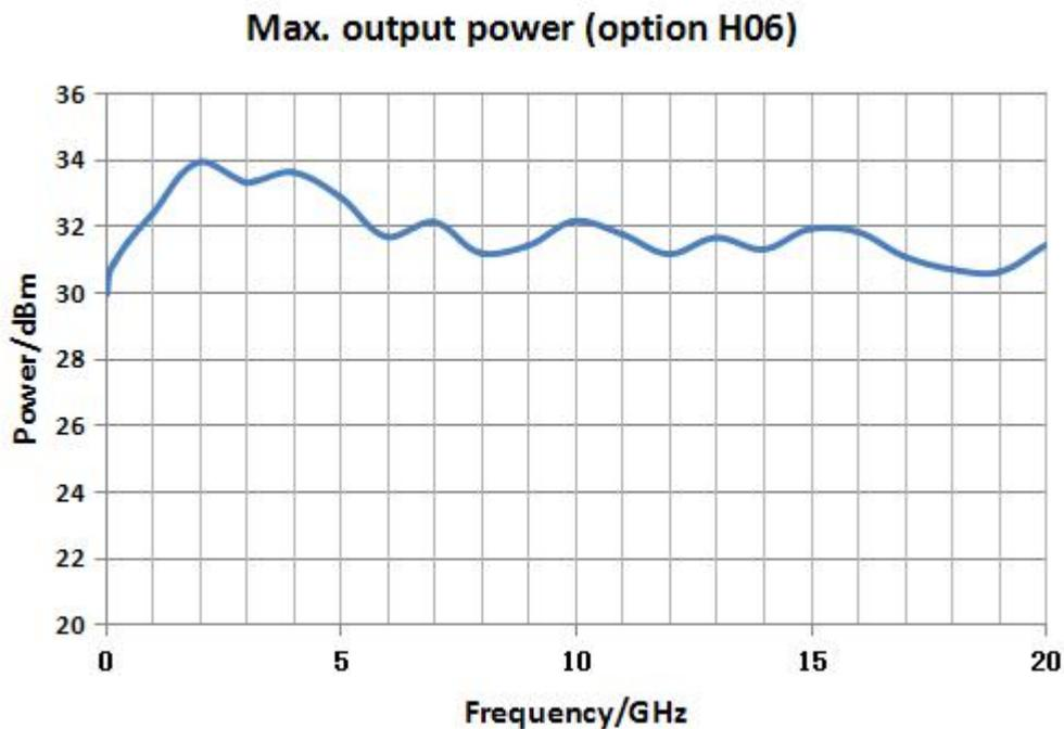
Fig.3.2 Max. Output Power of S1465D+H06
