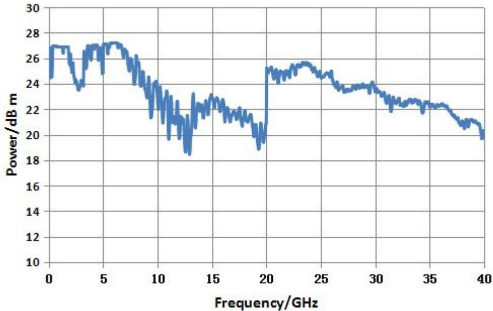
Fig.3.3 Max. Output Power of S1465F+H05
